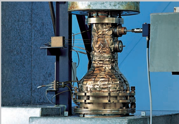
High temperature wind tunnel, 0.1 ... 80 m/s, +20 °C... +400 °C
